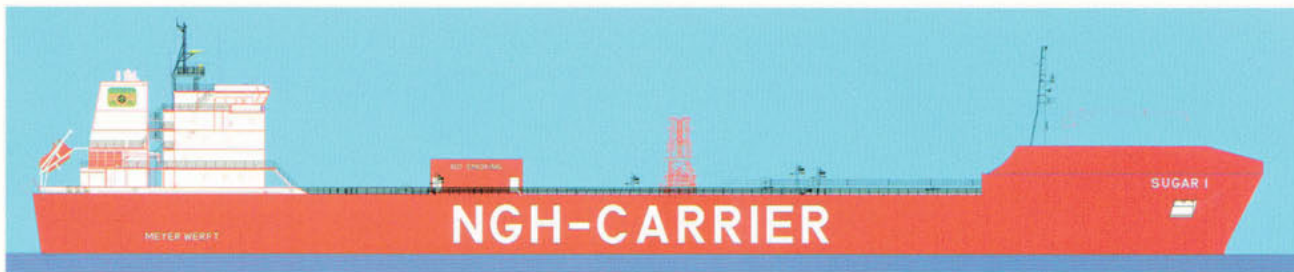
Side view of the Pellet Carrier (NGH-Carrier) specially designed by MEYER WERFT for the transportation of gas hydrate pellet cargo.
