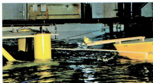
Testing the behaviour of the Pellet Carrier versus the behaviour of the Floating Production Unit during different sea states in the North Atlantic.
